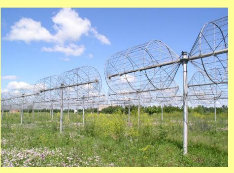
In UTR-2 observations three sections of the radio telescope with a total area of  $30000 \text{ m}^2$  were used. It provides the beam of  $1^{\circ}x13^{\circ}$ . Registrations were carried out with the DSP-Z (Digital Spectral Polarimeter) with high frequency (4 kHz) and time (100 ms) resolution.
