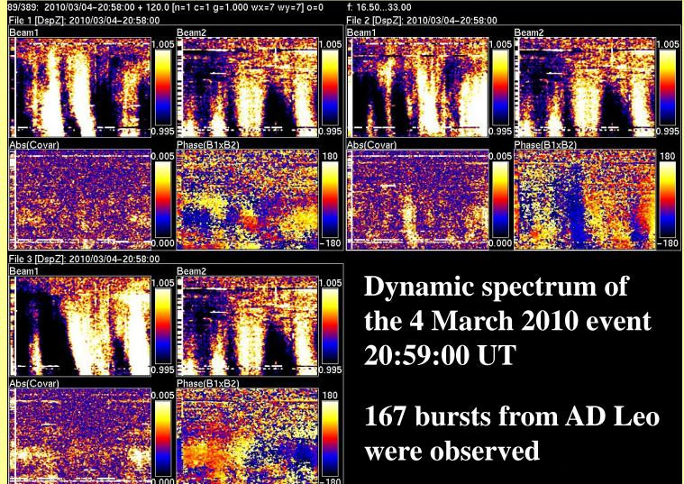
Three beams of the radio telescope were used (Beam 1, Beam 3 and Beam 5). For each beam we have 4 images – radio emission, which were received with the North – South antenna, radio emission, which were received with the East – West antenna, crossspectrum and phase spectrum of signal.
